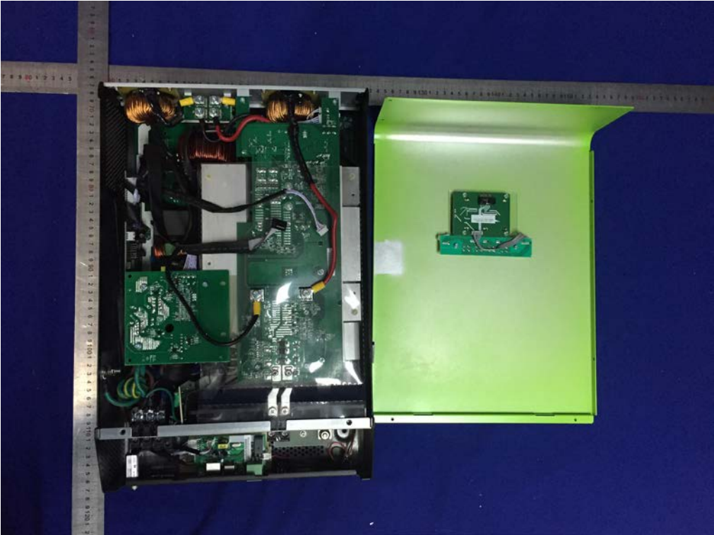
Fig. 24 -- FlinInfini Lite 3kW-48V&FlinInfini Lite 4kW-48V inside view I
